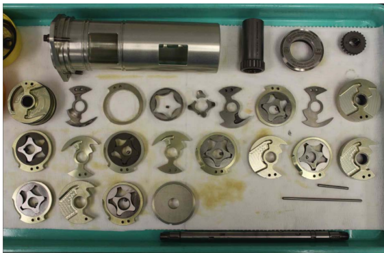
Figure 6: CH350's Oil Pump Component Breakdown.
