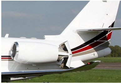
Figure 2: Deployed Bucket Type Thrust Reverser.
